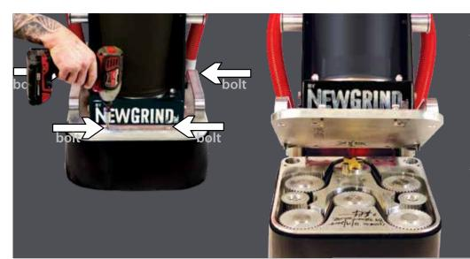
The Rhino is built with durability in mind – all machines are equipped with heavy duty extra wide drive belts for a low maintenance durable belt life. On the off chance a belt breaks, you can change it in less than 10 minutes right on your jobsite. This self-service feature is unique to our equipment, and it keeps the contractor's valuable time and money in mind.
